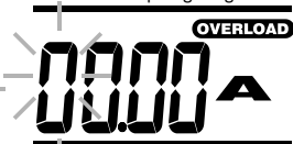
Overload Amperage Digits
